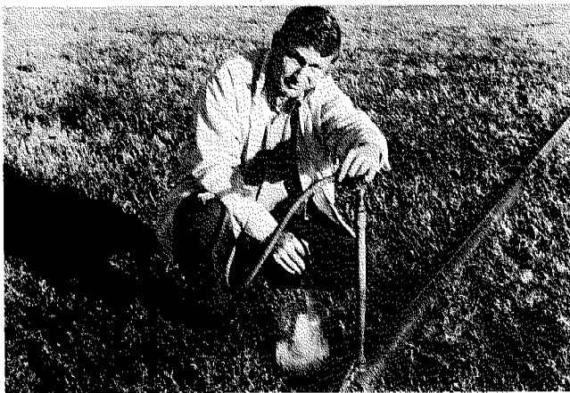
Figure 11-46.—Measuring sprinkler discharge using a hose to direct the water into a container.
