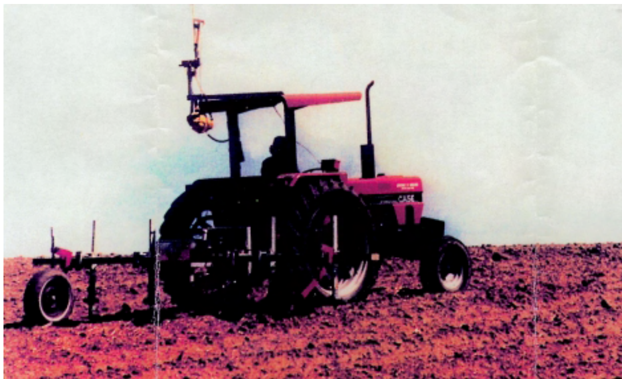
Figure 1 Mobile four-electrode sensing system
