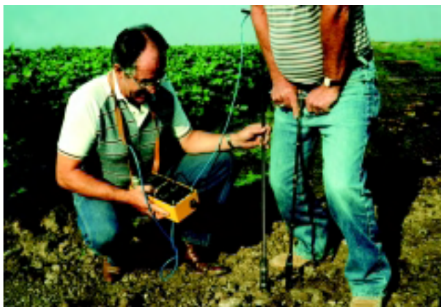
Figure 14–26 Monitoring salinity level of soil-moisture
