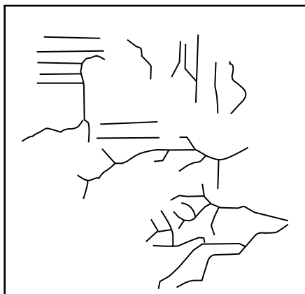
Figure 14-3 Extent of subsurface drainage for a field as shown by infrared photo and interpretive sketch (photo: Champaign County Soil and Water Conservation District and the Agricultural Engineering Department, University of Illinois)
