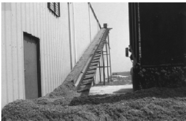
Figure 12–21 Heavy-duty alley gutter cleaner with chain drive (courtesy Patz Sales, Inc. and Husky Farm Equipment, Ltd.)
