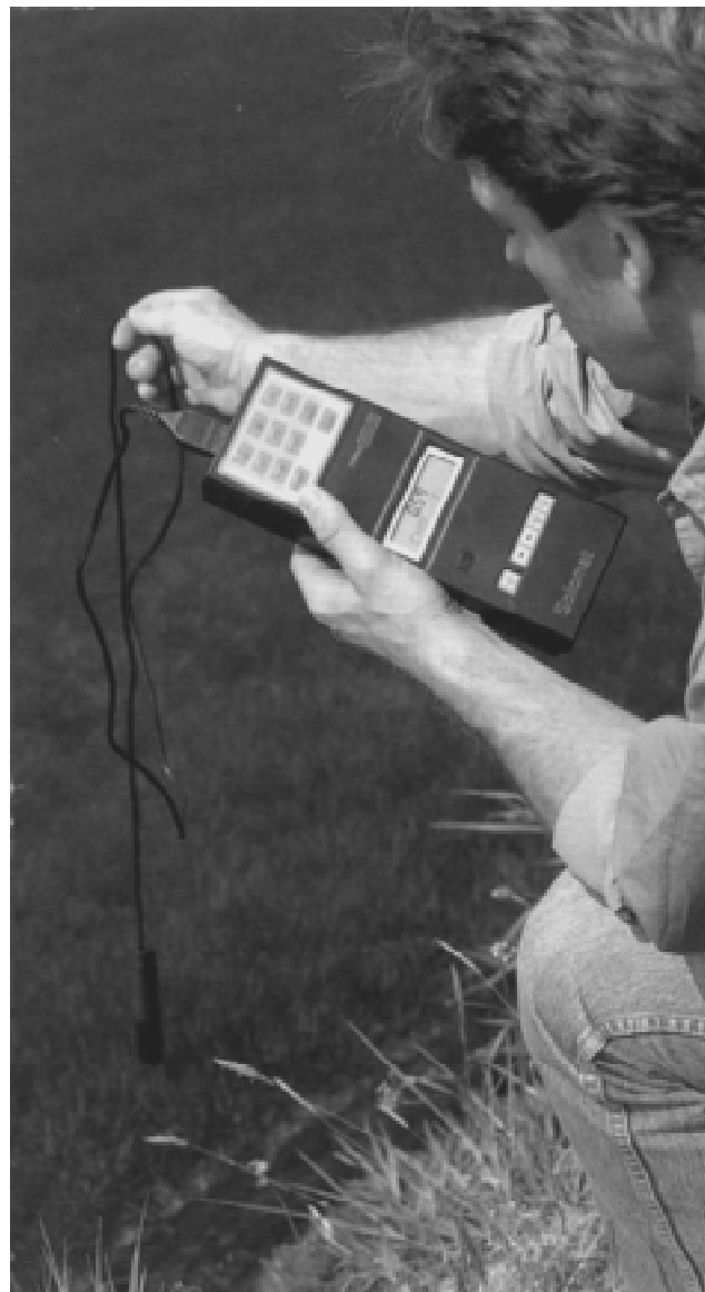
Figure 12-121 Water quality measurement electronically (courtesy Solomat Neotronics)
