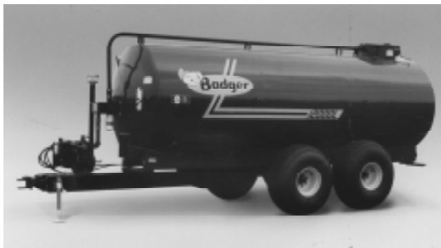
Figure 12-87 Separate pump load tanker spreader (courtesy Badger Northland, Inc.)
