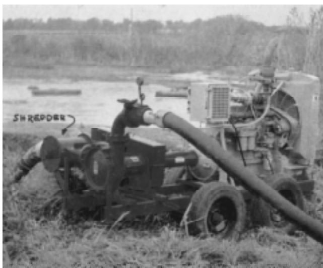
Figure 12–39 Cutter-shredder for slurry waste (courtesy Hydro Engineering, Inc.)
