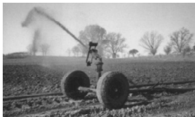
Figure 12–102 Traveling gun sprinkler with soft and hard hoses (courtesy Tuckasee Irrigation)
