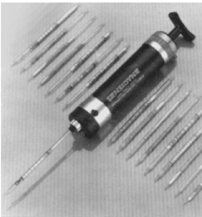
Figure 12–114 Air sampler with different gas detection tubes (courtesy Sensidyne, Inc.)
