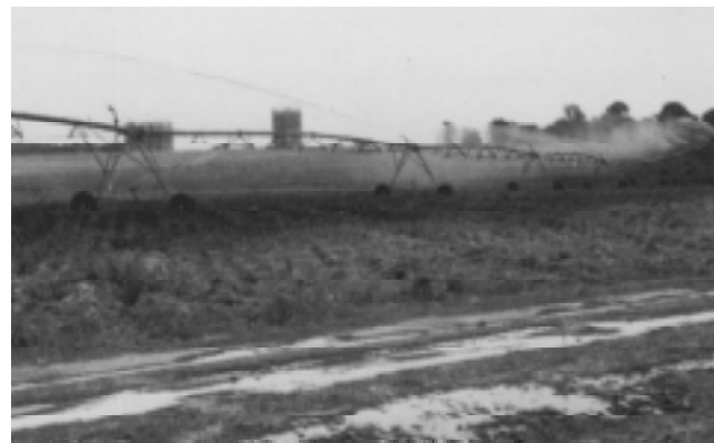
Figure 12–104 Center pivot sprinkler (courtesy of Hydro Engineering, Inc.)
