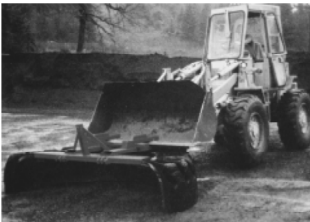
Figure 12–11 Tractor scraper blade using earthmover tire (courtesy Tillamook Concrete Groving)
