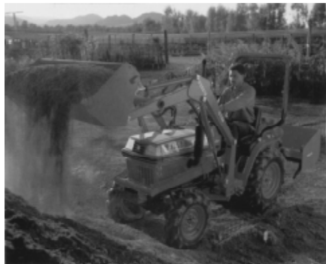
Figure 12–12 Lawn and garden tractor scraping equipment (courtesy Kubota Tractor Corporation)
