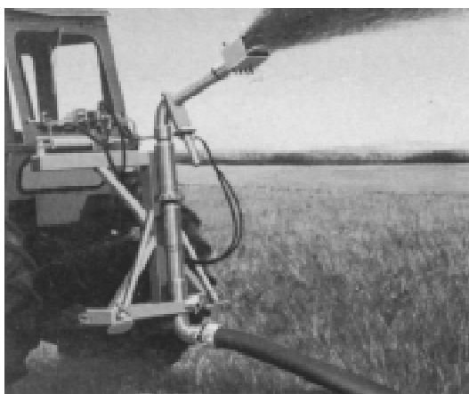
Figure 12-101 Stationary big-gun slurry sprinkler (courtesy Hydro Engineering and J. Houle & Fils, Inc.)
