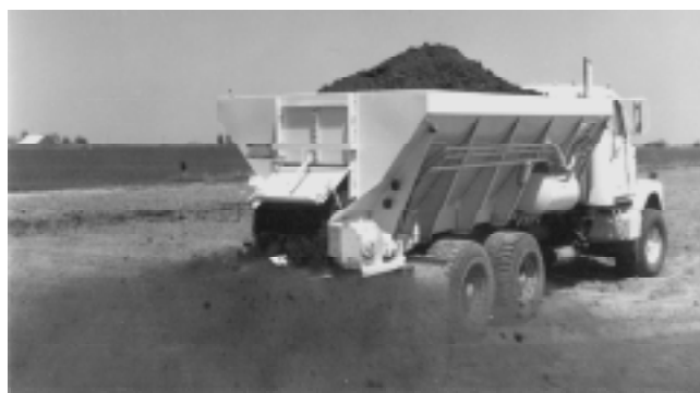
Figure 12–85 V-bottom rear-unload broadcast spreader (courtesy of Denair Trailer Company)
