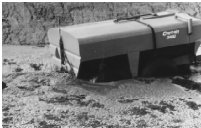
Figure 12–84 Conveyor self-loading waste spreader (courtesy Jerry's Iron Works)
