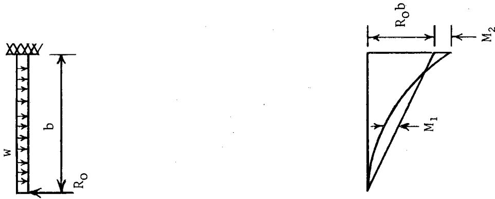
Figure 20. Effect of reactive support on moments.
