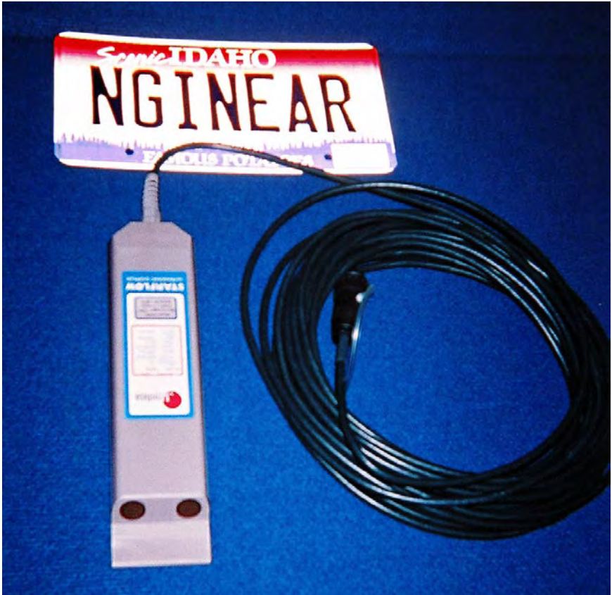
Photograph 1. The Unidata StarFlow ultrasonic Doppler flow meter contains a pressure transducer and two velocity sensors. The instrument is 11 inches in length, 2½ inches in width, and 1 inch in height. It can be installed facing upstream or downstream.
