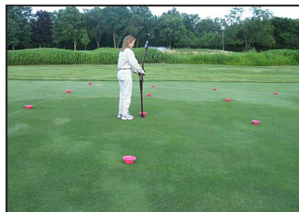
Figure 3. Sampling soil moisture with TDR300.
