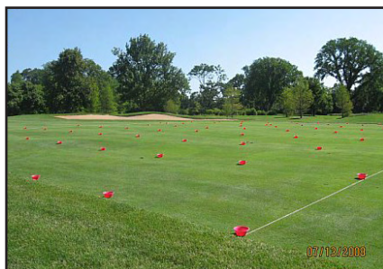
Figure 2. Catch cans laid out in 9 x 9 grid pattern.
